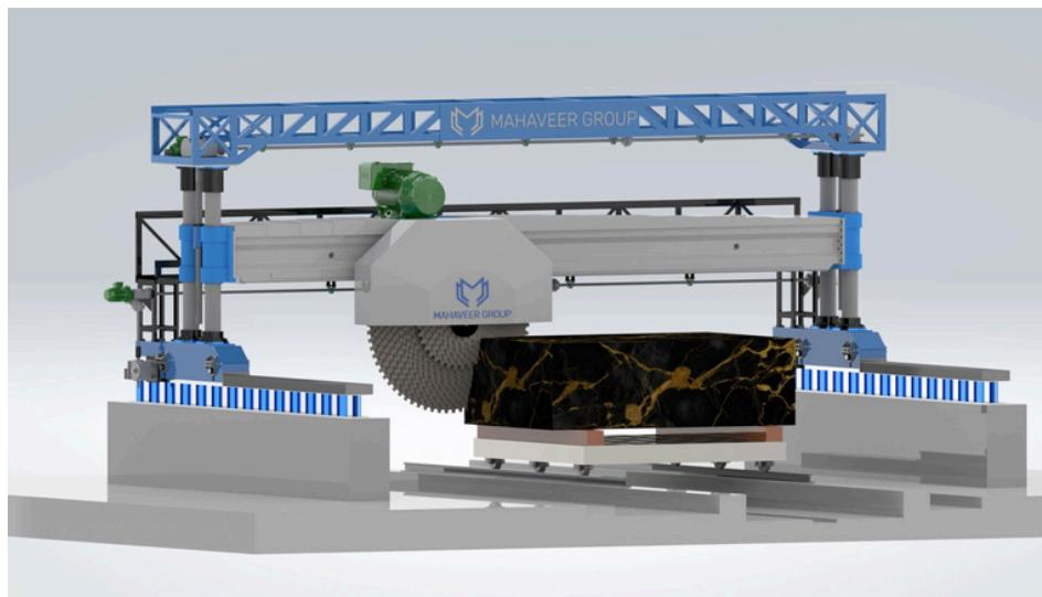
**Our MDPL-STC** is for multi blade block saw for cutting stone blocks into slabs of varying thickness.
