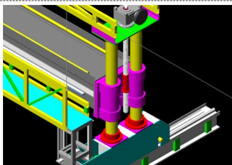
We are giving UP-DOWN movement on big diameter screw system. Both side of beam with reduction gearbox & motor for high accuracy & less maintenance
